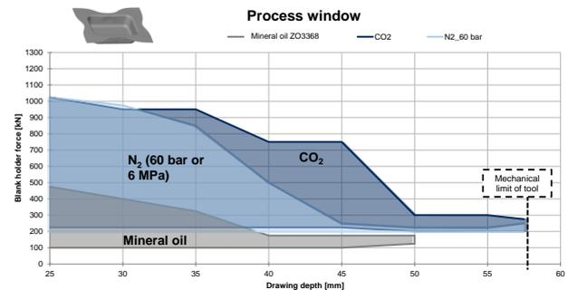
Figure 3: Process windows for deep drawing of a rectangular cup using different lubrication systems.
