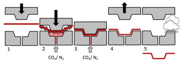
Figure 1: Process sequence of sheet metal forming using volatile media as lubricant substitute [2].
