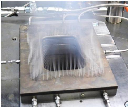
Figure 2: Free flow out of the CO<sub>2</sub> through laser-drilled microholes in the die of the deep drawing tool.
