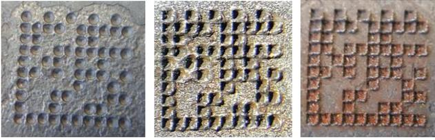
Figure 8: QR-Codes generated by needling (left), low resolution laser-engraving (middle) and high resolution laser engraving (right), all with successful optical recognition.
