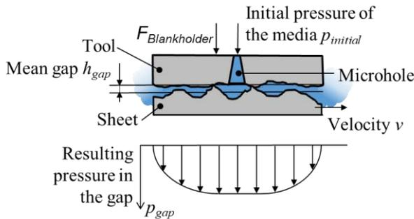
Figure 4: Schematic illustration of the resulting pressure between sheet and tool.
