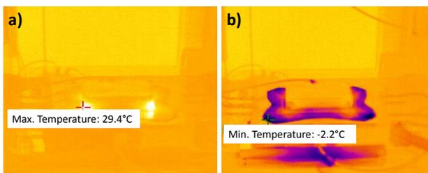
Figure 5: Measured temperature on the part surface after deep drawing using (a) nitrogen and (b) liquid carbon dioxide as volatile lubricant
