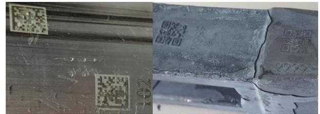
Figure 7: QR-Codes generated by fibre-laser: Aluminium at 550°C damaged by collisions (left); Steel at RT covered by an oxide-layer development at 900°C for three hours (right). All codes have been recognised successfully.
