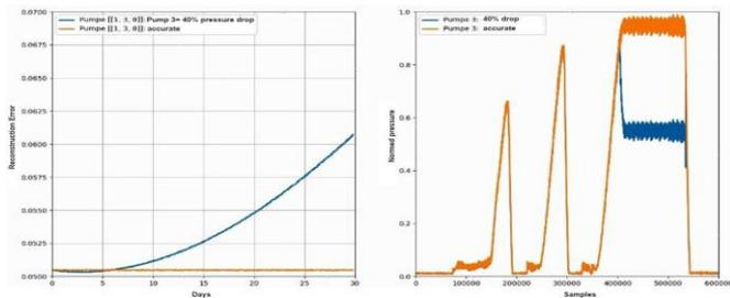
Fig. 9. Slinking deviation over time (blue, right) and normal behaviour (orange, right) and the model output (left).
