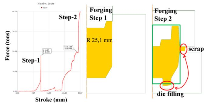
Fig. 6. Above: Finite element simulation of the forming process. Below: Result of parameter variation.
