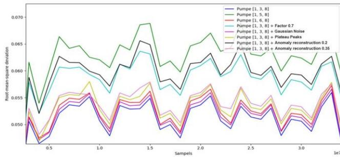
Fig. 8. Averaged reconstruction error over time sequences of the described anomaly scenarios.
