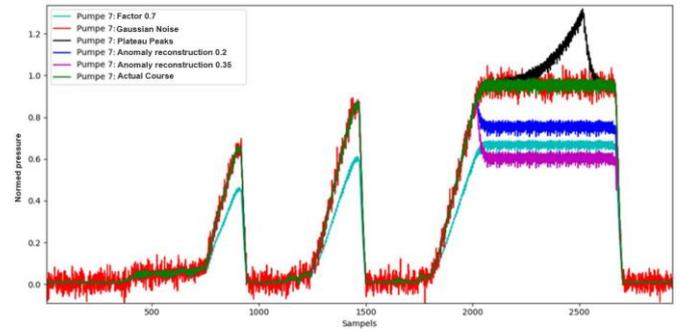
Fig. 7. Measured pressure (green), measured anomaly (violet) and artificial anomalies (other colours) of one cycle.
