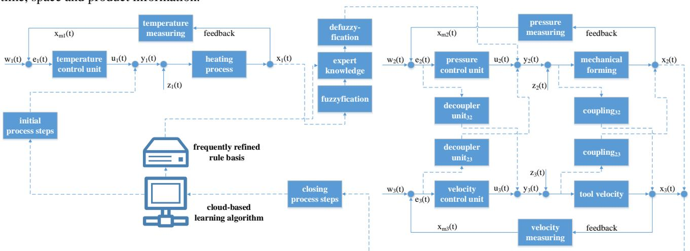
Fig. 4. Control logic and FIS: Example of heating and forming process with multiple inputs and outputs to the system.
