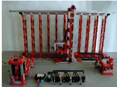
Figure 5. IAS High-bay Warehouse
